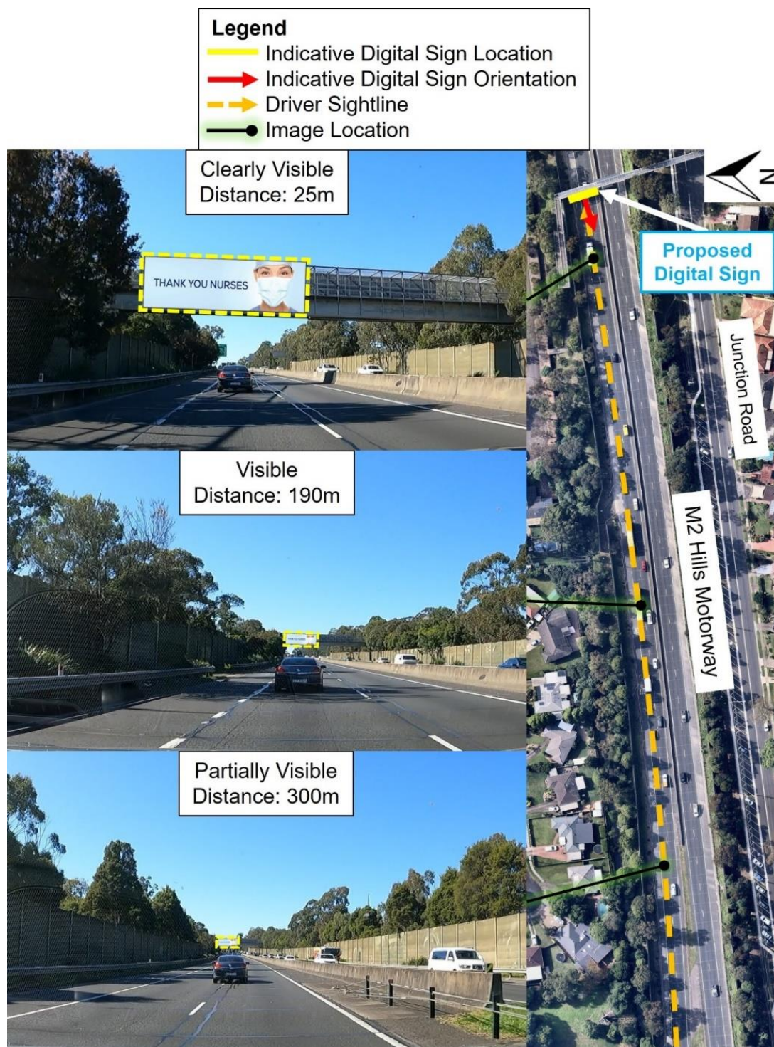
Figure 5.4: In-vehicle viewing range and views along the M2 eastbound
